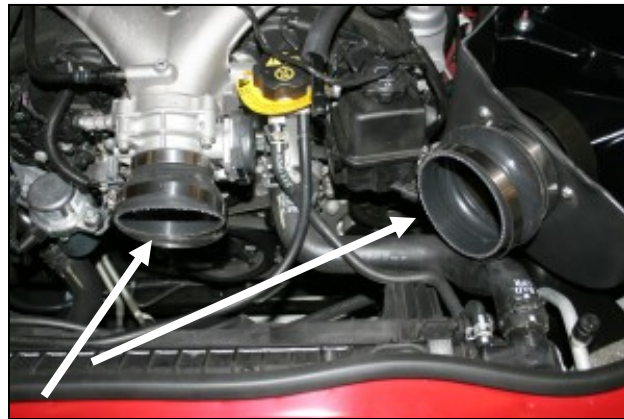
14. Install the hump hose (#7) onto the filter adapter using two #64 hose clamps (#22). Next install the reducing coupler (#5) with one #48 hose clamp (#21) on the throttlebody and one #64 hose clamp (#22) on the large end.
