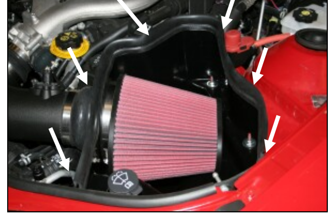
18. Install the Airaid Premium Filter (#1) onto the filter adapter and tighten the clamp. Next install the weather strip (#8) onto the top of the CAB. For ease of installation, start the front of the CAB near the radiator and work your way around towards the fender. Reinstall the engine cover and oil fill cap.
