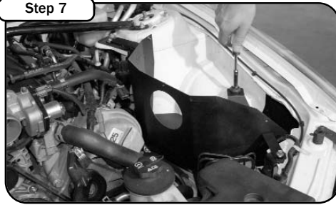
Step 7 Transfer the rubber isolation mount from the stock airbox to the housing. Position the housing into the engine bay. Re-install the 10mm bolts removed in steps 5 and 6.
