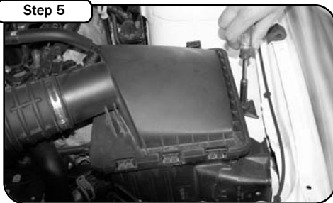
Step 5 Remove the 10mm screw that secures the airbox to the inner fender well. Save the bolt you will be re-using this bolt later. Remove airbox out of the engine bay.
