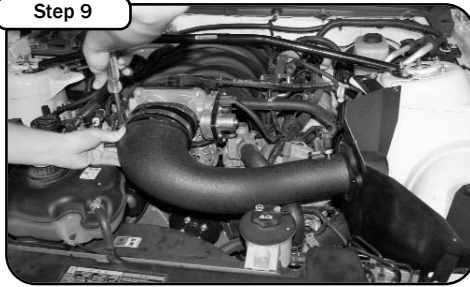
Step 9 Place coupler and hose clamps on the throttle body. Position tube into coupler and tighten the clamps down.
