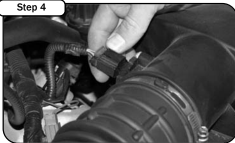
Step 4 Disconnect the MAF Sensor. you need to pull up on the red clip in order to remove the sensor.
