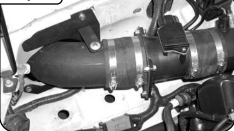
Attach tube assy. to cover plate bracket using (1) m6x16 mm screw, (1) lock washer and (2) sealing washers.
