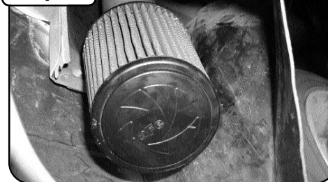
Install air filter from beneath. Access can be easier if inner fender splash panel is flexed out of the way for clearance. Be sure filter is clamped securely and check and re-tighten after a few hours of operation.
