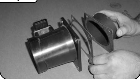
Install MAF adapter using gasket + (4) M6 x 16mm hex screws and lock washers.
