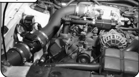
Place enclosed CARB EO sticker on a clean/smooth surface on or near the intake system. EO identification label is required in passing Smog Check inspection. Make sure all hoses and clamps are tight and that all electrical components are secure.
