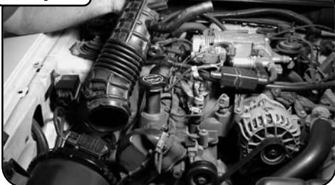
Loosen boot clamps at MAF sensor and throttle body. Disconnect vent tubes at boot and resonator box. Remove boot.
