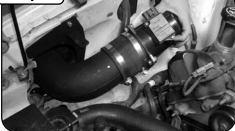
Install 3.5" dia. coupler on small end of filter tube and pass filter end thru fender well. Attach MAF sensor to coupler using 2 #056 clamps. Installation can also be done from below.
