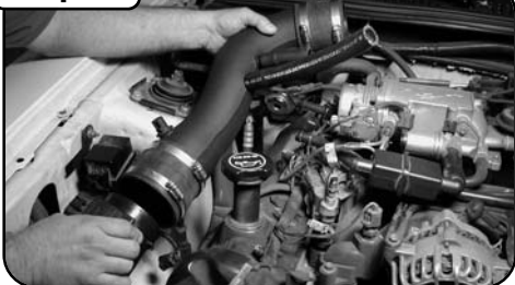
Place the 3.5" dia. Coupler over large end of "L" tube and 3" dia. Coupler over small throttle body end of tube. Attach large coupler end to MAF sensor. Using (2) #056 clamps swing tube assy. into position and attach to throttle body using (2) #048 clamps.
