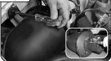
Remove 8mm head screw securing filter canister. Remove canister assy. by rotating up and out to clear snorkel from inner fender well. Place on workbench and remove MAF sensor from filter canister.
