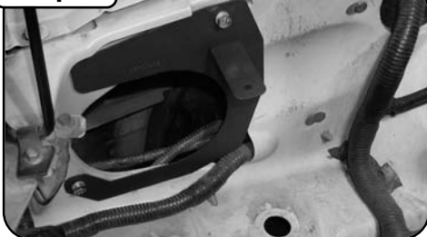
Install cover plate and bracket over snorkel hole in fender well. Use an m6 x 16 hex screw, flat washer, lock washer and nut at lower hole + screw and flat washer at upper location.
