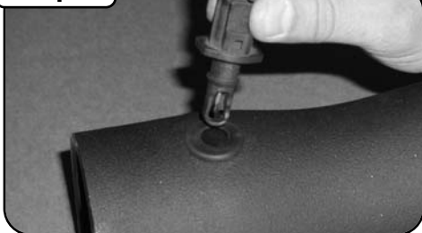
Install rubber grommet in hole on "L" tube. Insert temp sensor into grommet
