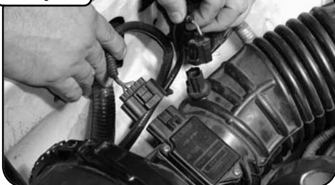
Disconnect wire harness from MAS airflow sensor (MAF) and disconnect temperature sensor. Remove temp sensor from boot.
